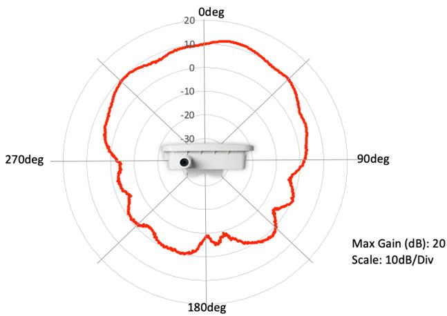
5 GHz Azimuth
