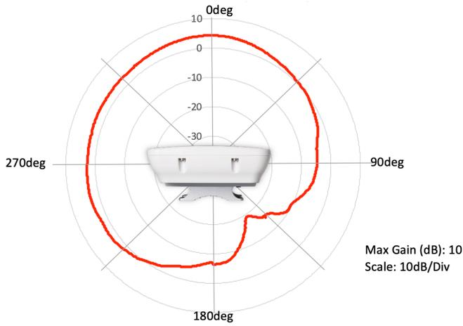
2.4 GHz Azimuth
