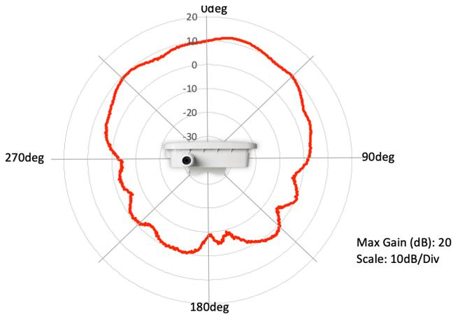
2.4 GHz Azimuth
