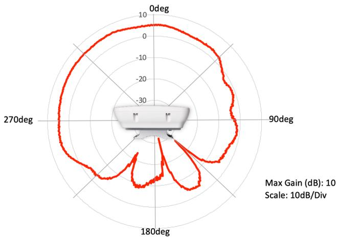
5 GHz Azimuth
