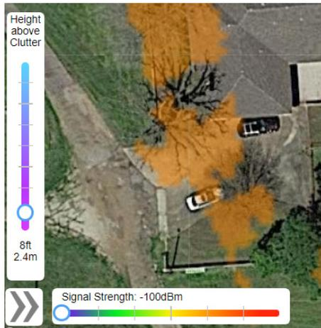
Height and Signal Strength sliders allow dynamic control of coverage for heat map.
